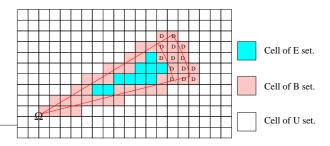
Fig. 8 A range-finder beam. The range finder is located at  $\Omega$  and its field of view is surrounded by red boundaries. It defines the three kind of cell types. The band, within the obstacle, lies is at the top right end of the field of view. Thus the cells marked with a "D" stand for cells where a detection event occurs.
