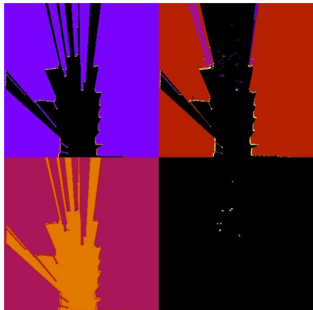
Fig. 9 Upper left: the observed map \mathcal{M}_o . Upper right: the static map \mathcal{M}_s . Bottom left: the difference map \mathcal{M}_d . Bottom right: the extracted foreground. For all the maps, the more hot is the color, the more positive is the value.
