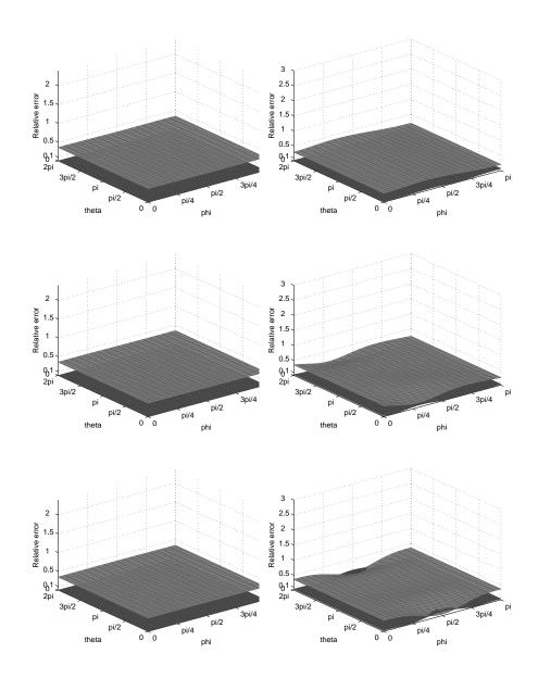
Figure 13: Relative error of the specific impedance for the DtN2 (black), the BGT2 (dark grey) for ka = 0.1 (left) and ka = 1 (right) for the incident angles  $\theta_0 = 0$  (up),  $\theta_0 = \frac{\pi}{4}$  (middle),  $\theta_0 = \frac{\pi}{2}$  (down).
