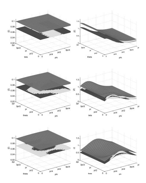
Figure 10: Absolute value of the specific impedance for the exact (clear grey), the DtN2 (black), the BGT2 (dark grey) for ka = 0.1 (left) and ka = 1 (right) for the incident angles  $\theta_0 = 0$  (up),  $\theta_0 = \frac{\pi}{4}$  (middle),  $\theta_0 = \frac{\pi}{2}$  (down).
