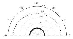
Figure 3: Absolute value of the specific impedance for the exact (solid), the DtN2 (crossed), the BGT2 (dashed).
