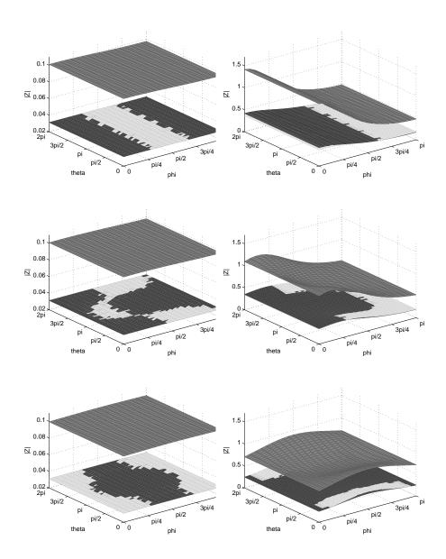
Figure 11: Absolute value of the specific impedance for the exact (clear grey), the DtN2 (black), the BGT2 (dark grey) for ka = 0.1 (left) and ka = 1 (right) for the incident angles  $\theta_0 = 0$  (up),  $\theta_0 = \frac{\pi}{4}$  (middle),  $\theta_0 = \frac{\pi}{2}$  (down).
