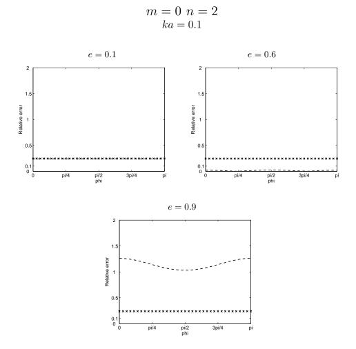
Figure 2: Relative error of the specific impedance for the DtN2 (crossed), the BGT2 (dashed).
