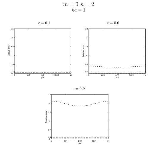
Figure 4: Relative error of the specific impedance for the DtN2 (crossed), the BGT2 (dashed).
