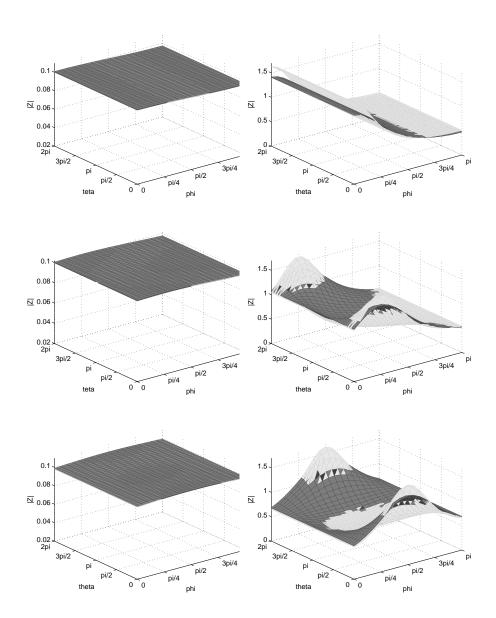
Figure 9: Absolute value of the specific impedance for the exact (clear grey), the DtN2 (black), the BGT2 (dark grey) for ka = 0.1 (left) and ka = 1 (right) for the incident angles  $\theta_0 = 0$  (up),  $\theta_0 = \frac{\pi}{4}$  (middle),  $\theta_0 = \frac{\pi}{2}$  (down).
