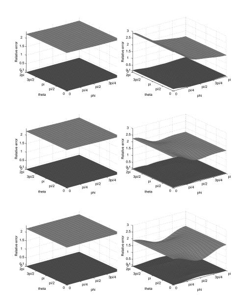
Figure 14: Relative error of the specific impedance for the DtN2 (black), the BGT2 (dark grey) for ka = 0.1 (left) and ka = 1 (right) for the incident angles  $\theta_0 = 0$  (up),  $\theta_0 = \frac{\pi}{4}$  (middle),  $\theta_0 = \frac{\pi}{2}$  (down).
