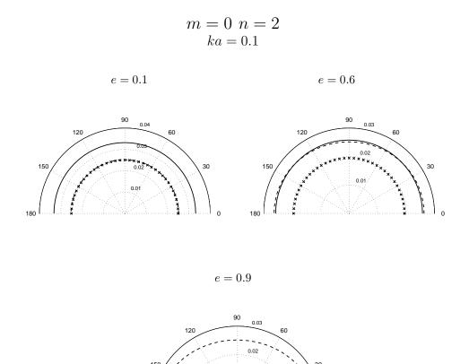
Figure 1: Absolute value of the specific impedance for the exact (solid), the DtN2 (crossed), the BGT2 (dashed).
