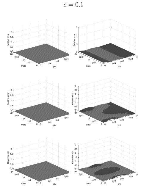
Figure 12: Relative error of the specific impedance for the DtN2 (black), the BGT2 (dark grey) for ka=0.1 (left) and ka=1 (right) for the incident angles  $\theta_0=0$  (up),  $\theta_0=\frac{\pi}{4}$  (middle),  $\theta_0=\frac{\pi}{2}$  (down).
