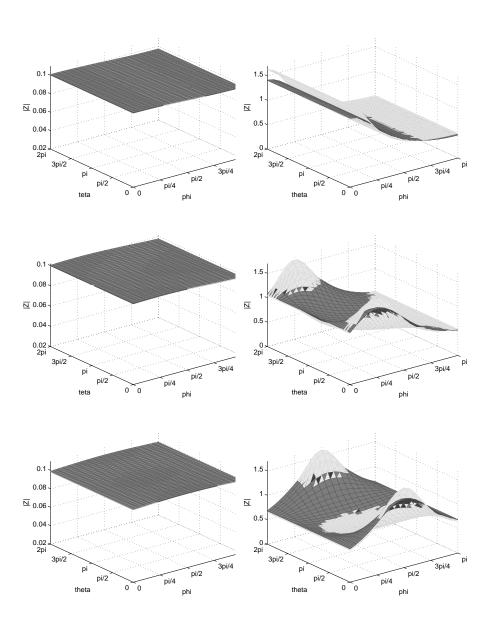
Figure 9: Absolute value of the specific impedance for the exact (clear grey), the DtN2 (black), the BGT2 (dark grey) for ka=0.1 (left) and ka=1 (right) for the incident angles  $\theta_0=0$  (up),  $\theta_0=\frac{\pi}{4}$  (middle),  $\theta_0=\frac{\pi}{2}$  (down).
