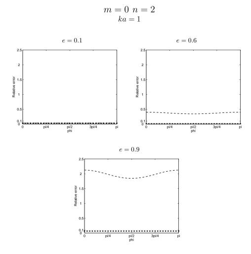
Figure 4: Relative error of the specific impedance for the DtN2 (crossed), the BGT2 (dashed).
