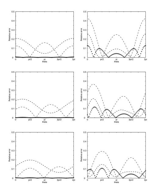
Figure 10: Relative error of the specific impedance for the DtN1 (dashed/dotted), the DtN2 (crossed), the BGT2 (dashed) for ka = 0.1 (left) and ka = 1 (right) for the incident angles  $\theta_0 = 0$  (up),  $\theta_0 = \frac{\pi}{4}$  (middle),  $\theta_0 = \frac{\pi}{2}$  (down).
