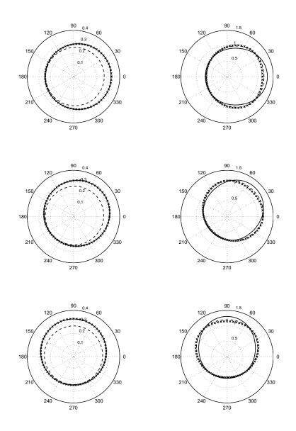
Figure 6: Absolute value of the specific impedance for the exact (solid), the DtN2 (crossed), the BGT2 (dashed) for ka = 0.1 (left) and ka = 1 (right) for the incident angles  $\theta_0 = 0$  (up),  $\theta_0 = \frac{\pi}{4}$  (middle),  $\theta_0 = \frac{\pi}{2}$  (down).
