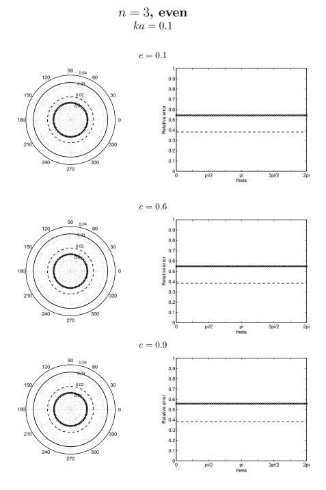
Figure 4: Absolute value (left) and relative error (right) of the specific impedance for the exact (solid), the DtN2 (crossed), the BGT2 (dashed).
