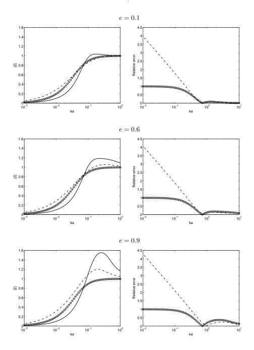
Figure 1: Absolute value (left) and relative error (right) of the specific impedance for the exact (solid), the DtN1 (dash), the BGT1 (circle).
