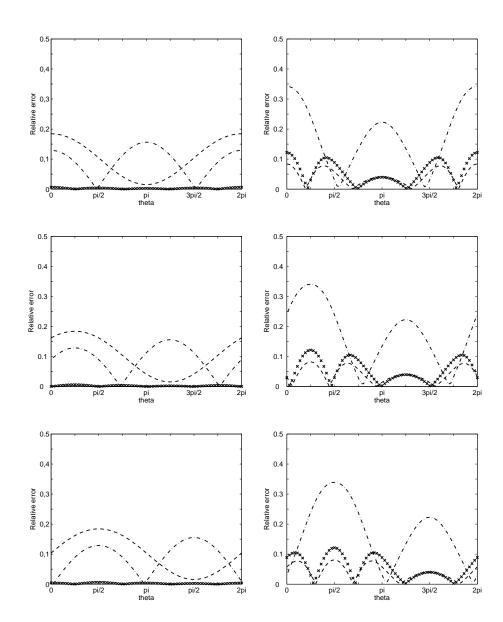
Figure 9: Relative error of the specific impedance for the DtN1 (dashed/dotted), the DtN2 (crossed), the BGT2 (dashed) for ka = 0.1 (left) and ka = 1 (right) for the incident angles  $\theta_0 = 0$  (up),  $\theta_0 = \frac{\pi}{4}$  (middle),  $\theta_0 = \frac{\pi}{2}$  (down).
