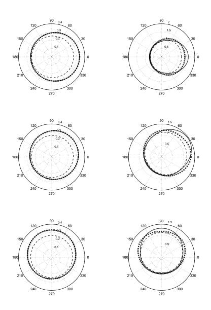
Figure 7: Absolute value of the specific impedance for the exact (solid), the DtN2 (crossed), the BGT2 (dashed) for ka = 0.1 (left) and ka = 1 (right) for the incident angles  $\theta_0 = 0$  (up),  $\theta_0 = \frac{\pi}{4}$  (middle),  $\theta_0 = \frac{\pi}{2}$  (down).
