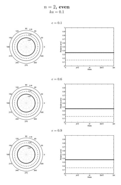
Figure 2: Absolute value (left) and relative error (right) of the specific impedance for the exact (solid), the DtN2 (crossed), the BGT2 (dashed).
