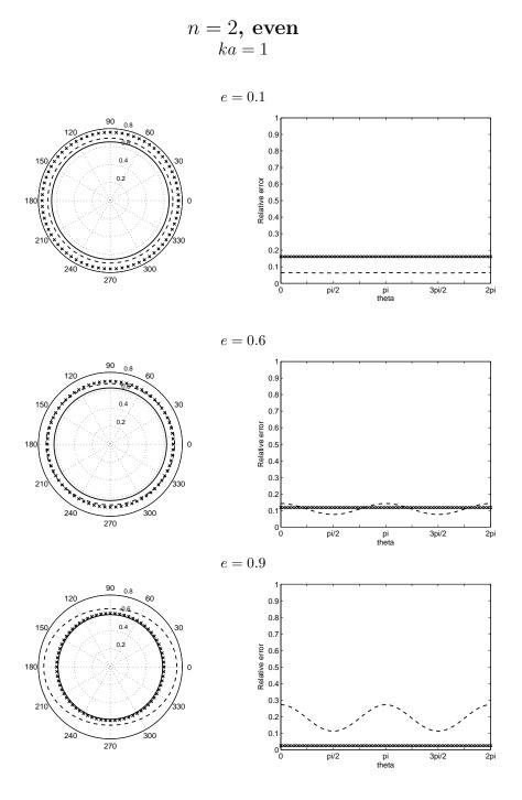
Figure 3: Absolute value (left) and relative error (right) of the specific impedance for the exact (solid), the DtN2 (crossed), the BGT2 (dashed).
