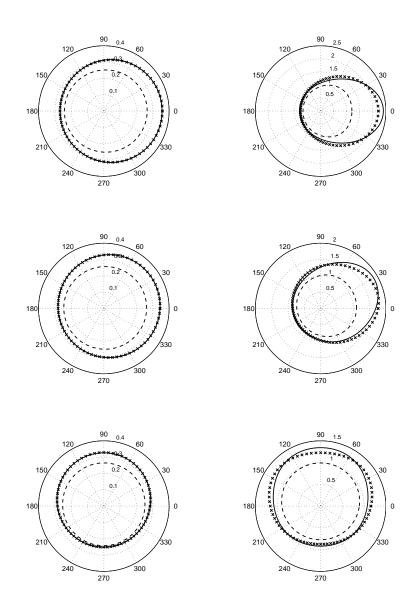
Figure 8: Absolute value of the specific impedance for the exact (solid), the DtN2 (crossed), the BGT2 (dashed) for ka = 0.1 (left) and ka = 1 (right) for the incident angles  $\theta_0 = 0$  (up),  $\theta_0 = \frac{\pi}{4}$  (middle),  $\theta_0 = \frac{\pi}{2}$  (down).
