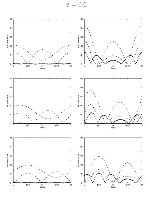
Figure 10: Relative error of the specific impedance for the DtN1 (dashed/dotted), the DtN2 (crossed), the BGT2 (dashed) for ka=0.1 (left) and ka=1 (right) for the incident angles  $\theta_0=0$  (up),  $\theta_0=\frac{\pi}{4}$  (middle),  $\theta_0=\frac{\pi}{2}$  (down).
