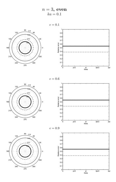
Figure 4: Absolute value (left) and relative error (right) of the specific impedance for the exact (solid), the DtN2 (crossed), the BGT2 (dashed).
