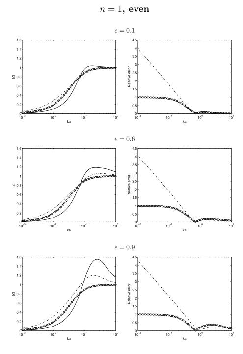
Figure 1: Absolute value (left) and relative error (right) of the specific impedance for the exact (solid), the DtN1 (dash), the BGT1 (circle).
