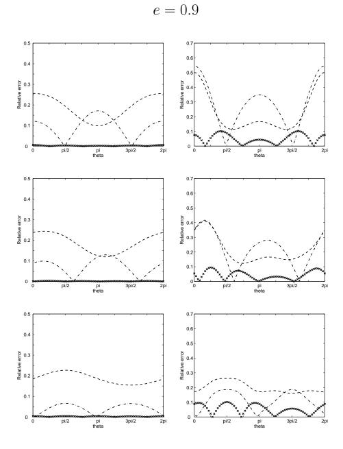
Figure 11: Relative error of the specific impedance for the DtN1 (dashed/dotted), the DtN2 (crossed), the BGT2 (dashed) for ka=0.1 (left) and ka=1 (right) for the incident angles  $\theta_0=0$  (up),  $\theta_0=\frac{\pi}{4}$  (middle),  $\theta_0=\frac{\pi}{2}$  (down).
