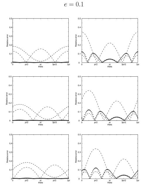
Figure 9: Relative error of the specific impedance for the DtN1 (dashed/dotted), the DtN2 (crossed), the BGT2 (dashed) for ka=0.1 (left) and ka=1 (right) for the incident angles  $\theta_0=0$  (up),  $\theta_0=\frac{\pi}{4}$  (middle),  $\theta_0=\frac{\pi}{2}$  (down).
