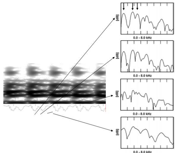
**Figure 1:** Principle of pitch synchronous amplitude adjustment. Left column: signal with pitch marks (bottom) and wide band spectrogram (top). Right column: four wide band spectra. The first three formants are indicated by arrows in the top spectrum.
