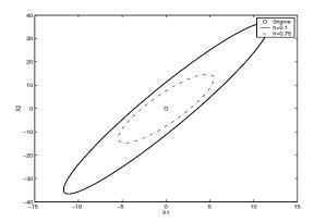
Figure 1: Ellipsoidal bounds on the domain of attraction
