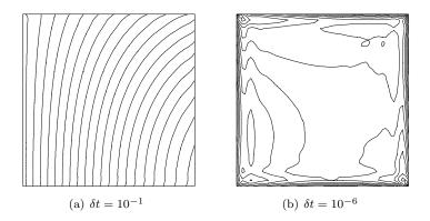
Figure 4: Pressure contour lines with  $\mathbb{P}_2/\mathbb{P}_2$  finite elements in a 40  $\times$  40 mesh:  $\pmb{u}_h^0=I_h^2\pmb{u}_0$
