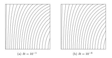
Figure 5: Pressure contour lines with  $\mathbb{P}_2/\mathbb{P}_2$  finite elements in a 40 × 40 mesh:  $\boldsymbol{u}_h^0 = P_h^2(\boldsymbol{u}_0, 0)$
