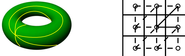
Figure 8: Left: invalid triangulation of \mathbb{T}^2 with a single vertex. Right: 9 periodic copies are shown.
