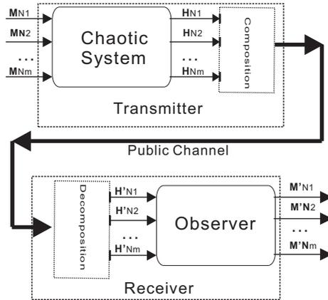
Figure 1: Scheme for multiple secure data transmission system
