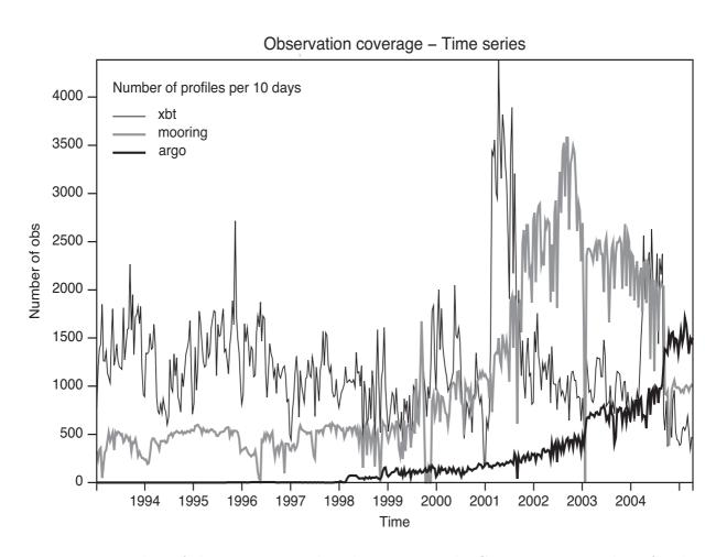
Figure 10: Number of observations used in the operational ECMWF ocean analysis for the XBTs, Moorings and Argo floats from 1993 to the beginning of 2005.
