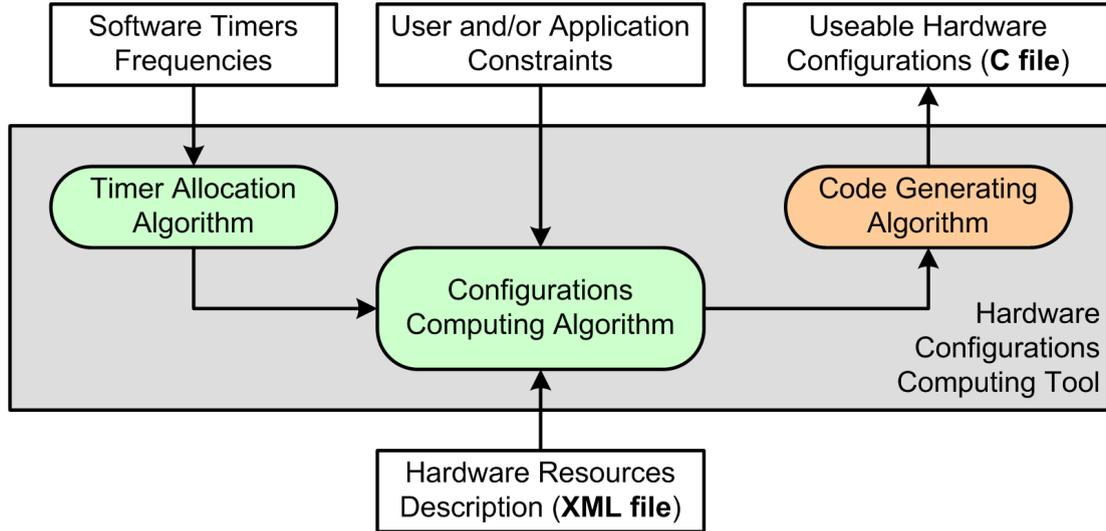
Figure 4.1: Detail of the hardware configurations computing tool
