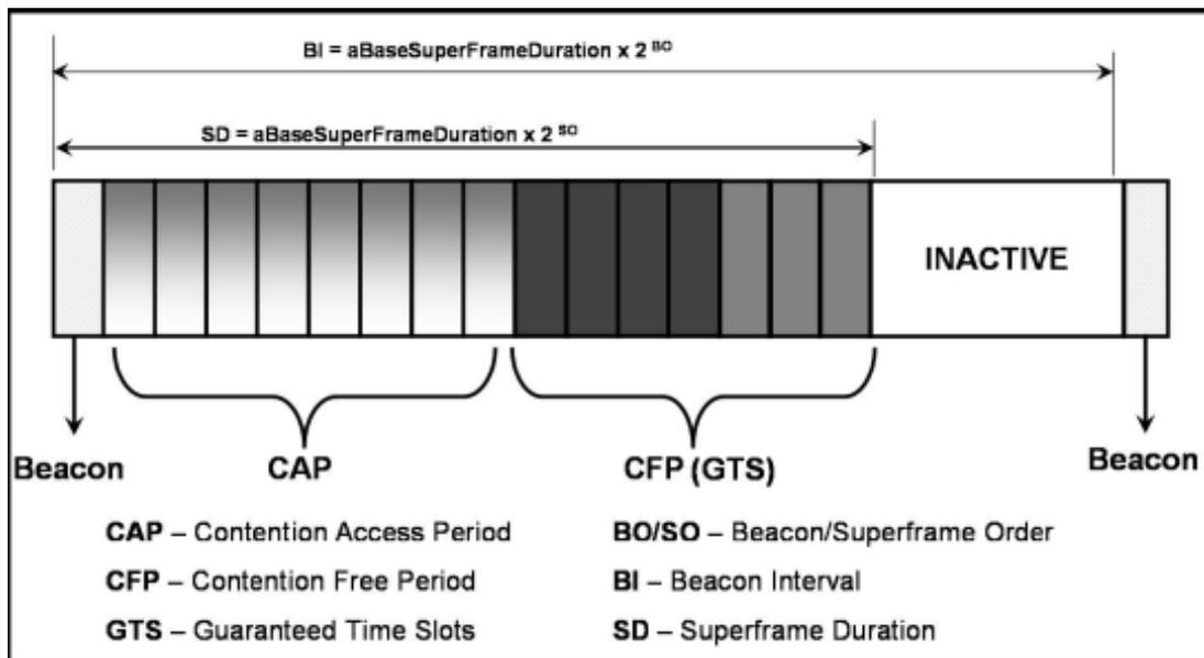
Figure 5.1: ZigBee superframe structure<sup>1</sup>
