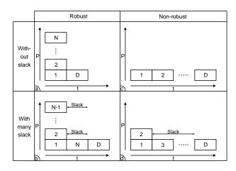
Fig. 9. Four schedules on P processors for different robustness and slackness, considering i.i.d. random variables and a join graph with N+1 tasks
