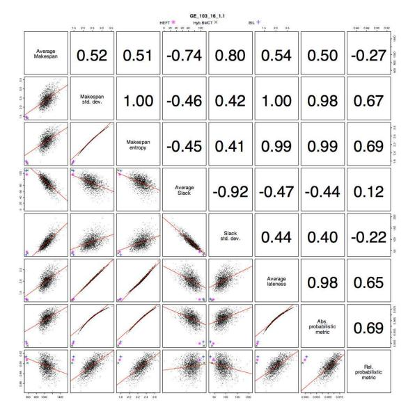
Fig. 5. Metrics correlation for a Gaussian Elimination graph of 103 tasks on 16 processors and UL=1.1. Lower part of the matrix: plot for 2000 random schedules and the 3 schedules given by BIL, HEFT and Hyb.BMCT heuristics. Upper part of the matrix: value of the Pearson coefficients for the random schedules.
