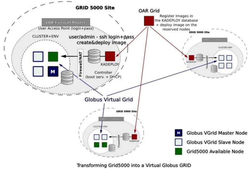
Figure 5: Globus Virtual Grid on Grid5000
