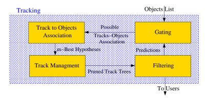
Figure 11: Architecture of multi-object tracking system
