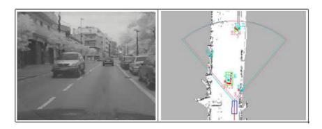
Figure 8: Moving object detected from laser data is confirmed by radar data.
