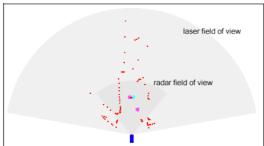
Figure 2: Left: the DaimlerChrysler demonstrator car. Right: an example of sensor data, laser measurements are displayed in small red dots and radar measurements displayed as bigger dots.
