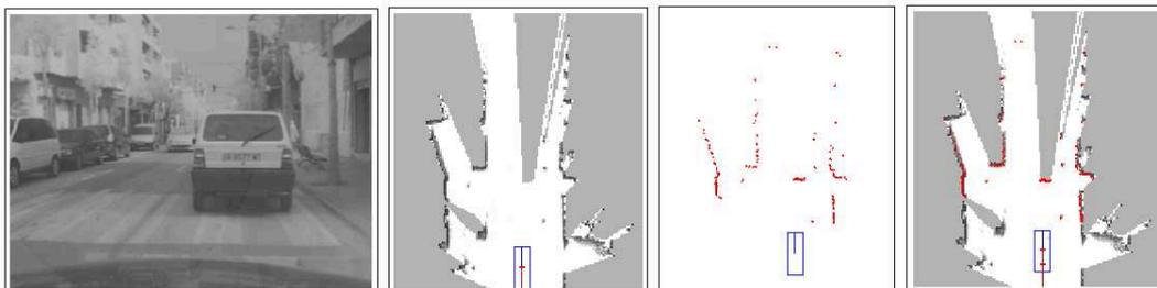
Figure 6: An example of scan matching. From left to right: reference image; map constructed so far  $M_{t-1}$  with previous vehicle location  $x_{t-1}$ ; new laser measurement  $z_t$ ; and matching result is obtained by trading off the consistency of the measurement with the map and the previous vehicle pose.
