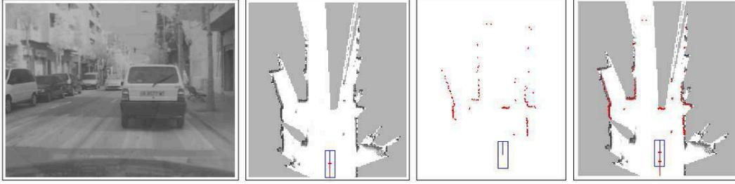
Fig. 6. An example of scan matching. From left to right: reference image; map constructed so far  $M_{t-1}$  with previous vehicle location  $x_{t-1}$ ; new laser measurement  $z_t$ ; and matching result is obtained by trading off the consistency of the measurement with the map and the previous vehicle pose.
