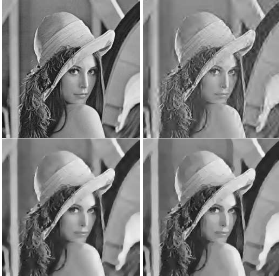
Figure 1: Example of image decompression - TL : Original image - TR : Compressed image using Daubechies 9-7 wavelet transform (the quantization coefficients are chosen by hand to outline the model features) - BL : Solution of (2.17) using \mu = 0.01 - BR : Solution of (2.17) using \mu = 0.001
