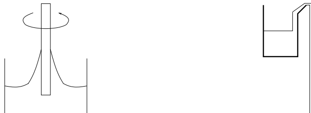
Figure 2: Schematic representation of two unexpected, counterintuitive behaviors for some polymeric fluids: the rod-climbing effect (left) and the open syphon effect (right).
