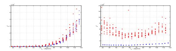
Figure 9: **Beam** - Test values. Safe (blue) and damaged (red) cases. X-axis: Thermal constraint. Y-axis: Test values. Left: Original  $\chi^2$ -test in Equation (14). Right: New  $\chi^2$ -test in Equation (22).
