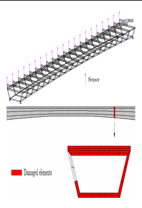
Figure 1: **Bridge deck** - Top: The model with the sensors location. Bottom: The damaged area.
