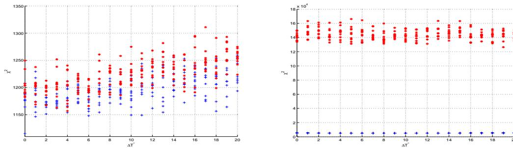
Figure 4: **Bridge deck** - Test values. Safe (blue) and damaged (red) cases. X-axis: Temperature variation. Y-axis: Test values. Left: Original  $\chi^2$ -test in Equation (14). Right: New  $\chi^2$ -test in Equation (22).
