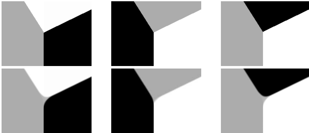
Figure 3: Junction evolution through AMSS. Top: three examples of grey level distribution over a triple point. Bottom: corresponding evolution. As noted in [3], this evolution depends on the ranking of the grey levels. Corners corresponding to level sets evolve in the same way as in Section 3.1. Since we are interested in identifying repeated angles in different views, the approach is still valid provided the possible contrast change is non-decreasing (and thus preserving the local grey level ranking of multiple junctions.)
