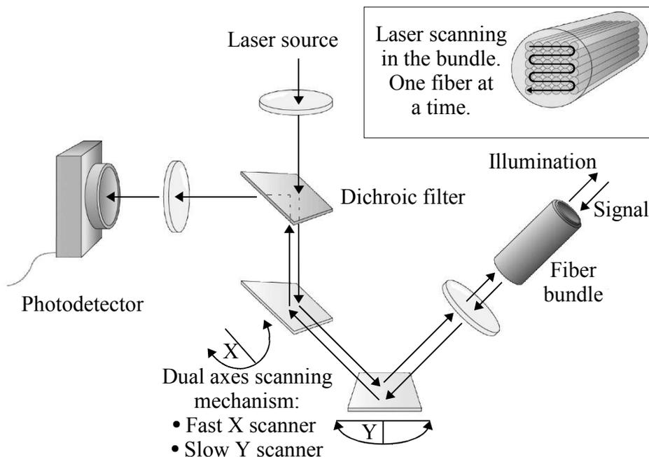
Fig. 1. Schematic principle of fibered confocal microscopy.
