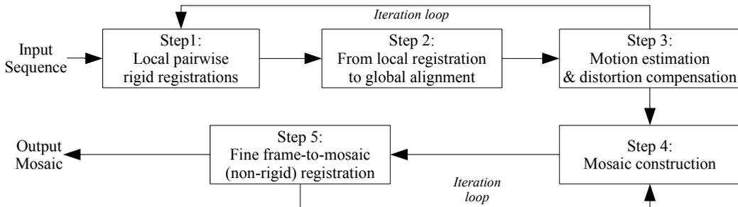
Fig. 8. Block diagram of the mosaicing algorithm.
