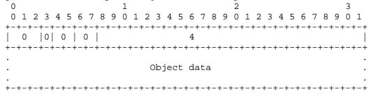
Figure 4: Compound Object Example with no Meta-Data.
