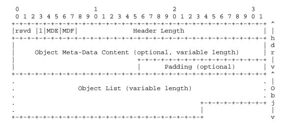
Figure 2: Carousel Instance Object Format
