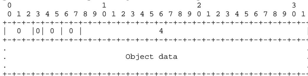
Figure 4: Compound Object Example with no Meta-Data.
