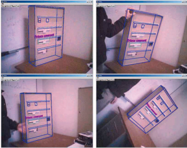
Fig. 5. Tracking of an electrical panel: The sequence features partial occlusions and large motion of both the camera and of the object.
