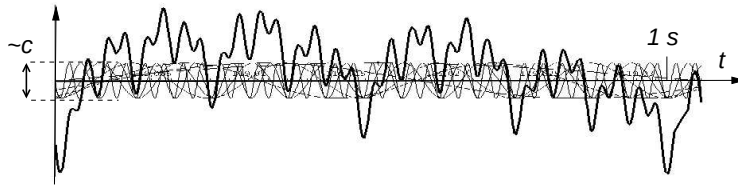
Figure 6: Temporal course over one second of the multi-sinus stimulus (19) and of its sinusoidal components. The amplitude of each sinusoidal component is proportional to contrast c .
