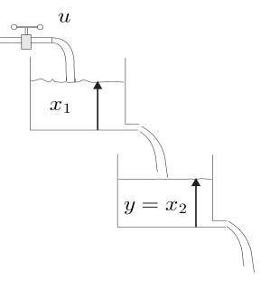
Figure 14: A two tank system
