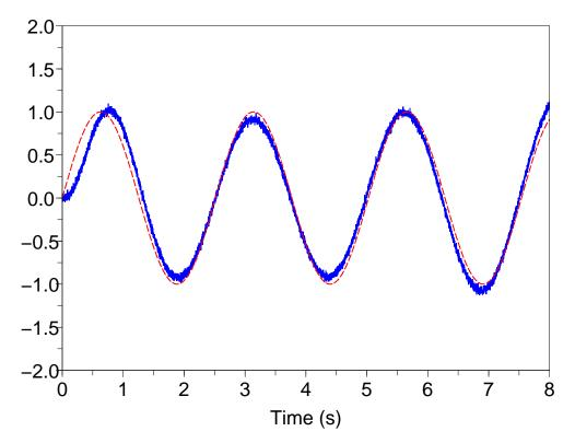
Figure 18:  $y^{\star}(t)$  (- -) and y(t) (-) with perturbation attenuation
