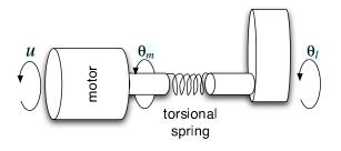
Figure 1: A single link flexible joint manipulator
