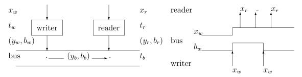
A simulation model of the LTTA To model an LTT architecture in Signal, we consider two data-processing functions that communicate by writing and reading values on an LTT bus. In Signal, we model an interface of these functions that exposes their (limited) control. The writer accepts an input  $x_w$  and defines the boolean flag  $b_w$  that is carried along with it over the bus.
