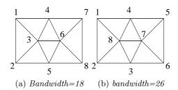
Fig. 2. A simple example of bandwidth with respect to nodes order.
