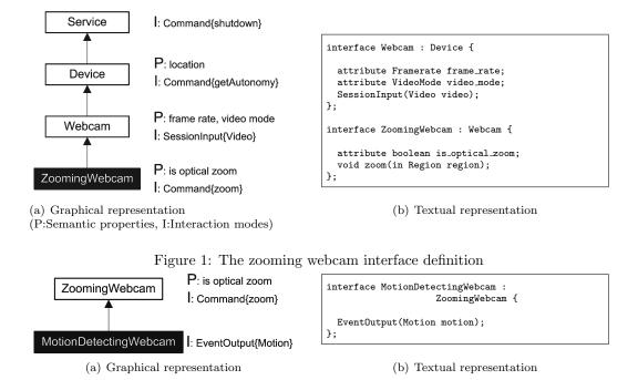
Figure 2: The motion detecting webcam interface definition
