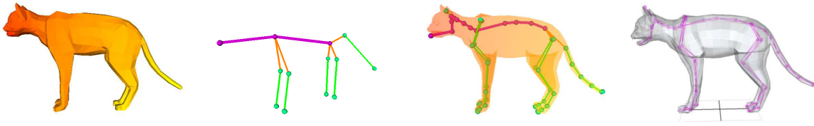
Figure 2: From left to right: a cat model, the computed harmonic graph with its symmetry axis, the computed harmonic skeleton compared to a previously handmade animation skeleton.
