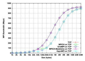
Figure 6: Comparison of MPI bandwith of the different MPI implementations on a distant network (grid) after TCP tuning
