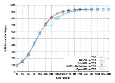
Figure 5: Comparison of MPI bandwidth of the different MPI implementations on a local network (cluster) with the default parameters
