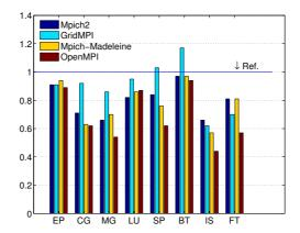
Figure 11: Relative comparison between the different MPI implementations on 2-2 nodes between two clusters, Ref. is MPICH2
