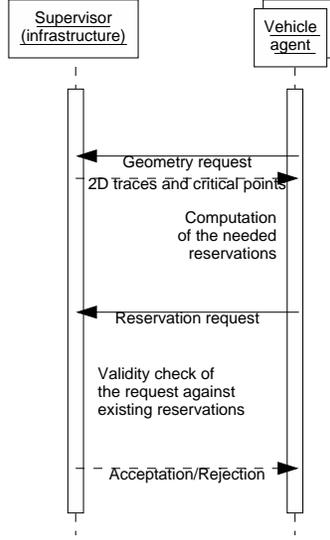
**Fig. 2.** A synopsis of the communications between a reservation agent and the crossroads supervisor. The proposed reservation scheme heavily relies on information exchanges between the supervisor and vehicles.
