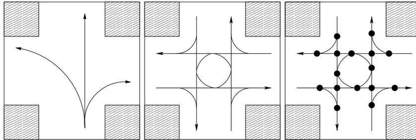
**Fig. 1.** A regular crossroads. Left: each vehicle entering it has three possibilities to get out. Center: trajectories that vehicles are able to, and *may*, follow. Right: only a small subset of critical points on the trajectories is where the risk of collision exists.
