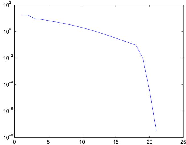
Figure 13: Steady NSE, Cavity B, Re=400, N=63. Residual vs iterations
