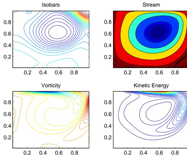
Figure 12: Steady NSE, Cavity B,  $Re=400$ ,  $N=63$ ; Isovalues for the streamfunction, the vorticity, the pressure and the kinetic energy
