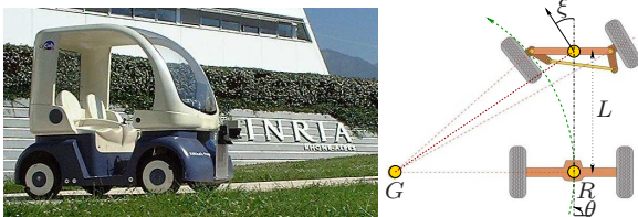
Fig. 5. The Cycab vehicle and its kinematics.
