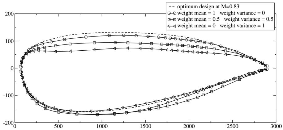
Figure 23: Comparison of the wing shape at the root section: optimum design at nominal Mach number and robust designs from the Pareto front.
