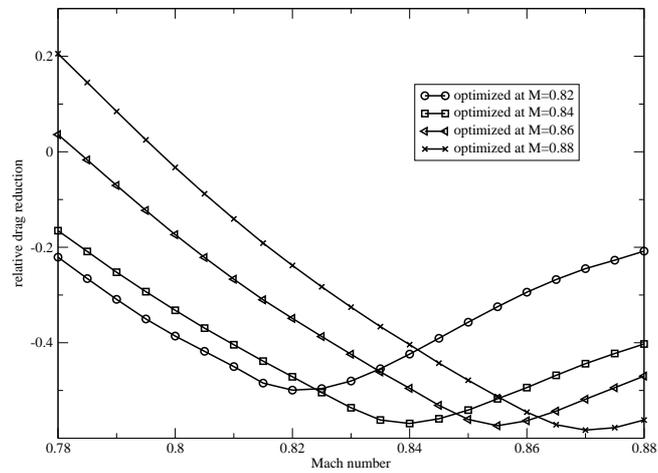
Figure 9: Relative drag reduction for a wing shape optimized at different Mach number values.
