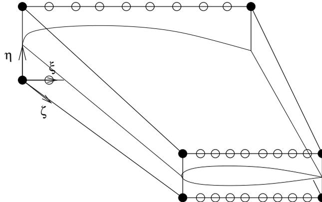
Figure 4: Example of FFD lattice around a wing.
