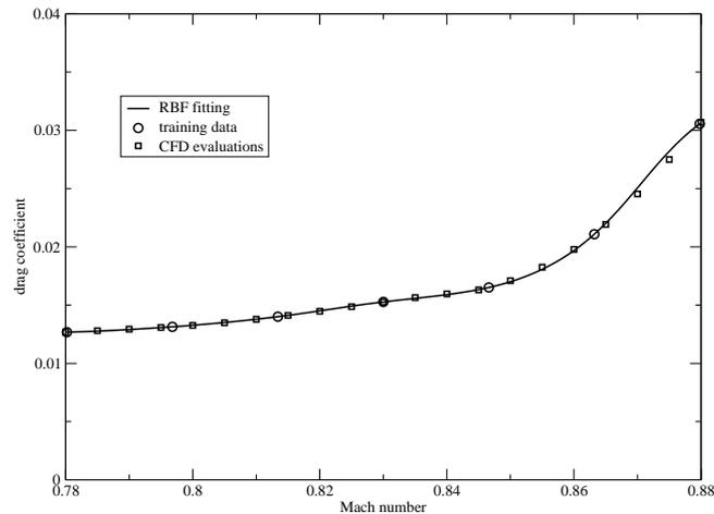
Figure 21: Seven-point fitting using RBFs for the robust design.
