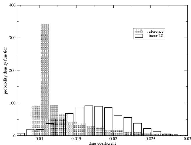
Figure 12: Probability density function of the drag coefficient: reference result compared to linear fitting.
