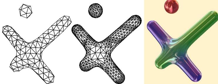
$\approx 180$  particles,  $\approx 350$  mechanical triangles, 3 skel. elements,  $\alpha_r = 32^\circ$
