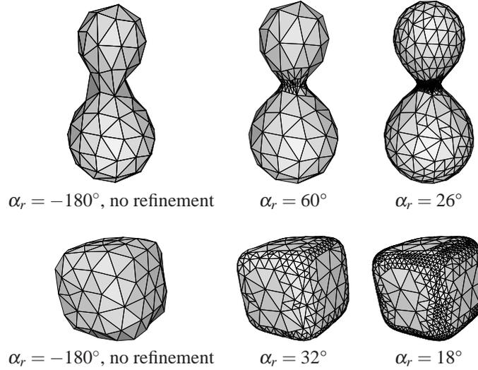
Figure 9: Results of geometry refinements with varying  $\alpha_r$ .
