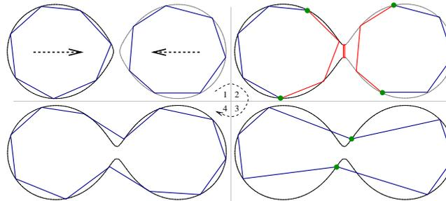
Figure 11: Summary of blending algorithm. *Stage 1:* At time  $t_{i-1}$ , the two surfaces are separated. *Stage 2:* At time  $t_i$ , the two geometric meshes collide (red). The corresponding mechanical triangles and their neighbors are marked for deletion (red). *Stage 3:* Marked triangles are deleted, and border points (green) are welded together. The geometric mesh is re-generated. *Stage 4:* At time  $t_{i+1}$ , the ALTERMESH() procedure subdivides the stretched edges.
