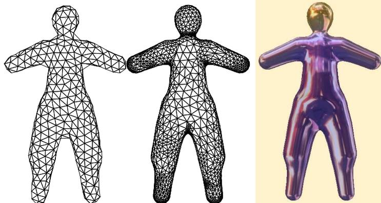
$\approx 530$  particles,  $\approx 1050$  mechanical triangles, 12 skel. elements,  $\alpha_r = 37^\circ$
