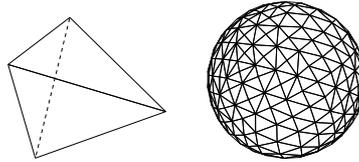
Figure 10: Geometric refinement on an extremely coarse mesh: although the metaball is mechanically represented by only four triangles (*left*), the refinement with  $\alpha_r = 20^\circ$  gives a well detailed mesh (*right*).
