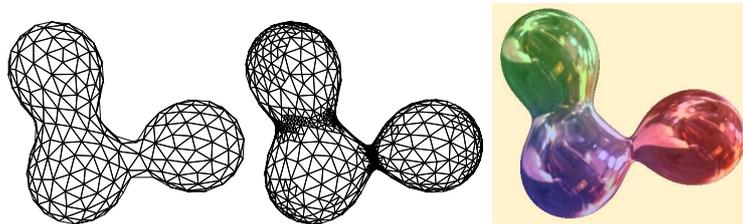
$\approx 350$  particles,  $\approx 690$  mechanical triangles, 3 skel. elements,  $\alpha_r = 26^\circ$
