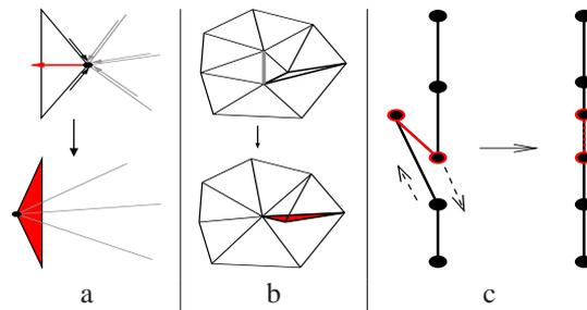
Figure 7: (a) Inversion resulting from a discrete integration. At time  $t$ , the gray forces are stronger than the black ones and push the point inside the triangle. At time  $t + dt$ , the point is pushed too far, resulting in an inversion. (b) Inversion resulting from collapsing the gray edge: the bold triangle becomes inverted (red). (c) Forces can create wrinkles that give inverted triangles when projected to the surface (red).
