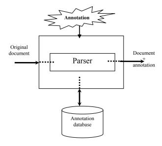
Figure 1: Architecture of generalized annotation system
