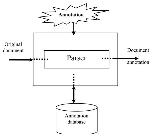
Figure 1: Architecture of generalized annotation system
