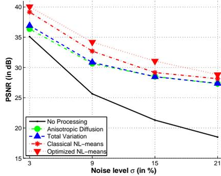
**Fig. 2.** PSNR values for the three compared methods for different levels of noise. The PSNR between the noisy images and the ground truth is called “No processing” and is used as the reference for PSNR before denoising. For each level of noise, the optimized NL-means algorithm outperforms the Anisotropic Diffusion method, the Total Variation method, and the classical NL-means.
