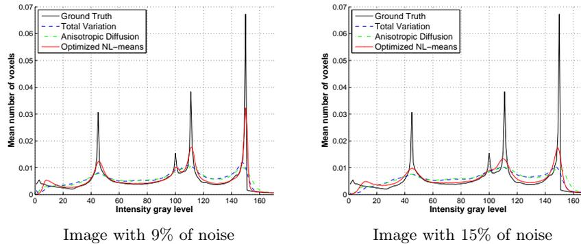
**Fig. 3.** Histograms of the restored images and of the ground truth. The histogram of the NL-means restored image clearly better fits to the ground truth one. Left: image with 9% of noise, Right: image with 15% of noise.
