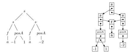
Fig. 2. Generation of relative positions from the labelled representation and maximal subterm sharing in memory.
