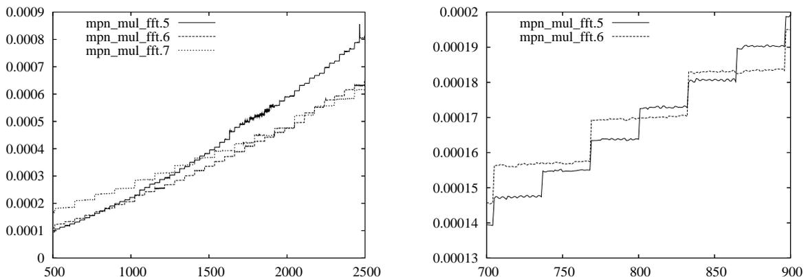
FIGURE 2. Time in seconds needed to multiply two numbers modulo  $2^n + 1$  with an FFT of length  $2^k$  for  $k = 5, 6, 7$ . On the right, the zoom (with only  $k = 5, 6$ ) illustrates that two curves can cross each over several times.
