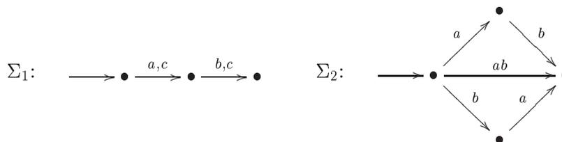
Figure 8: The synchronous systems  $\Sigma_1$  and  $\Sigma_2$  are both weakly endochronous and weakly isochronous, but  $\Sigma_2$  is not endochronous because the independent operations  $a$  and  $b$  can be executed in any order
