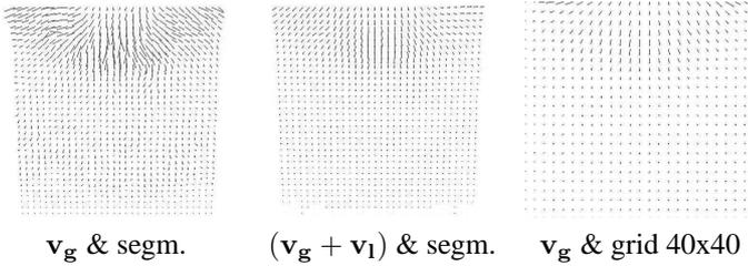
**Fig. 3.** Local vs global motion, with and without segmentation
