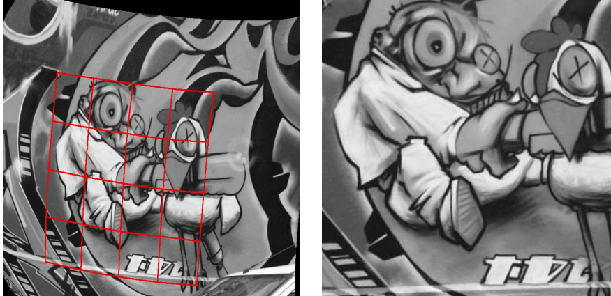
Figure 3: Visual tracking with the second-order minimization. The image on the left shows the transformation of the regular grid after 40 images of the sequence. The image on the right shows that the warped area of interest in the reference frame is equal to the reference template.
