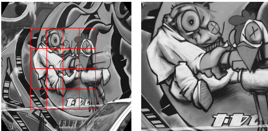
Figure 1: Case study for testing the proposed approach and comparing the convergence rate of minimization algorithms. The image on the left shows the regular grid defining the area of interest in the first image. The image on the right shows the corresponding template.
