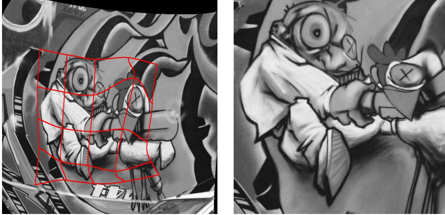
Figure 2: Visual tracking with the Gauss-Newton minimization. The image on the left shows the transformation of the regular grid after 40 images of the sequence. The registration fails due to the real-time constraints. This is clearly visible in the right image where the warped area of interest in the reference frame is not equal to the reference template.
