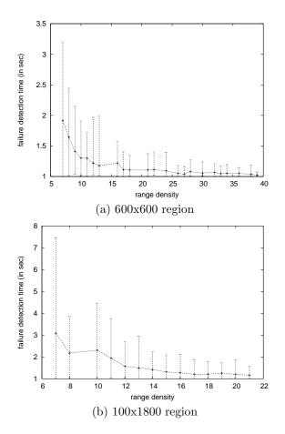
Figure 1: Failure detection time vs. range density
