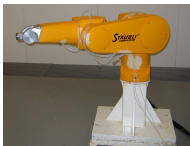
Figure 7: Flat configuration of a Stäubli Rx90
